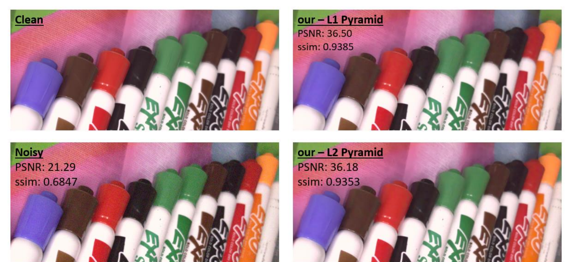
L1-Pyramid vs L2-Pyramid loss functions over SIDD image example
