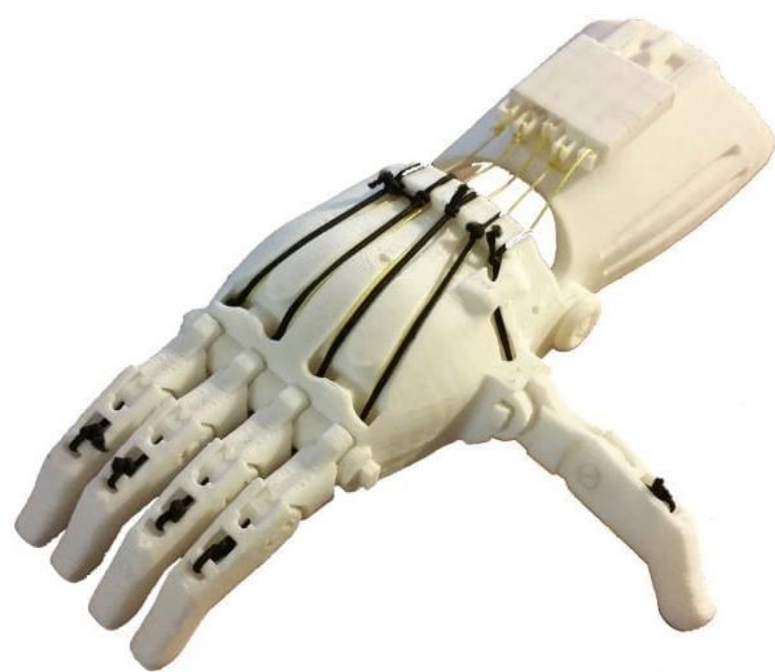
A 3D-printed prosthetic hand by e-Nable
